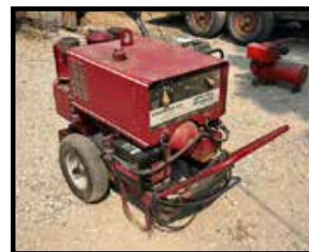
Portable Lincoln 225DC arc welder w/auxiliary power
