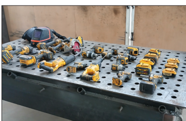
Welding Down Draft Table/Tools
